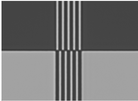
Fig. 6: 200nm dense lines/space pattern (400nm pitch) obtained in transmitted light at 248nm using water immersion for resolution enhancement
