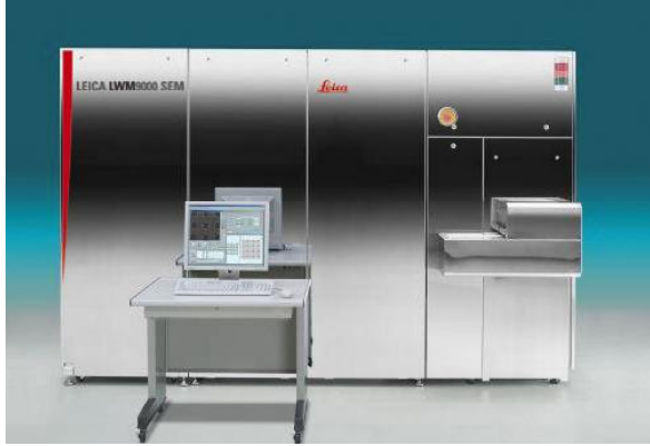
Fig. 3: The LWM9000 SEM with the manual (non-SMIF) loading system
