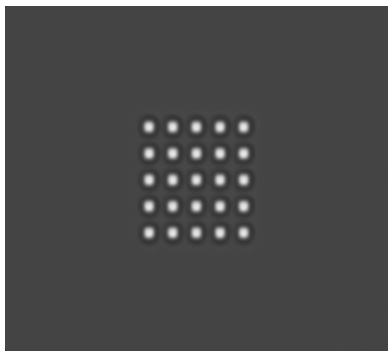
Fig. 7: Dense array of 300nm contacts on binary mask obtained in transmitted light on the LWM500 WI
