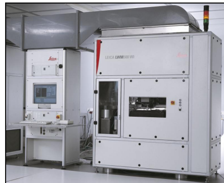
Fig. 2: The optical based LWM500 WI in the new temperature- controlled mini-environment.
